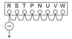
• Never test the withstand voltage on the inverter.
