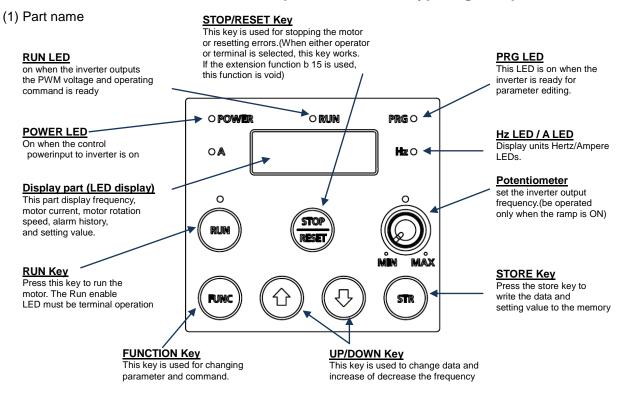
Fig.4-1 LED Type Digital Operator
