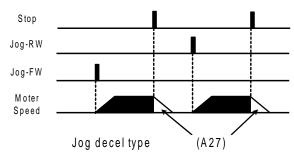
0:Free-run stop 1:Deceleration stop 2:DC injection braking
