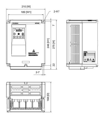
(2) N700E-150LF/185LFP, N700E-185LF/220LFP, N700E-220LF, N700E-150HF/185HFP, N700E-185HF/220HFP, N700E-220HF/300HFPmodel external dimension.(mm)
