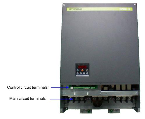
Fig1-6Front cover removed
