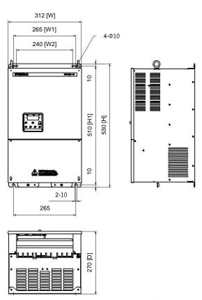
(3) N700E-300HF/370HFP, N700E-370HF/450HFPmodel external dimension.(mm)
