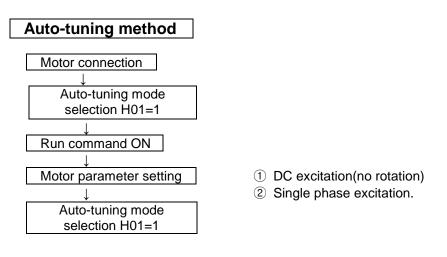
End display Auto-tuning process completed :-- o<sup>+</sup>
