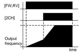
•When the terminal is turned off, the equipment is turned off, the equipment is returned to the original acceleration and deceleration time (F02 acceleration time1 and F03 deceleration time1). UseA54 (acceleration time2) and A55 (deceleration time2) to set the second stage acceleration and deceleration time.
