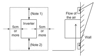
Ensure proper spacing for ventilation to prevent the unit from overheating.
