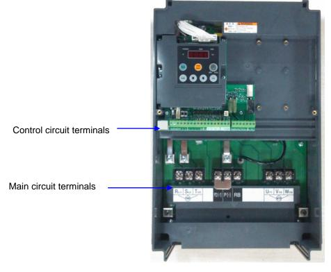
Fig1-4 Front cover removed
