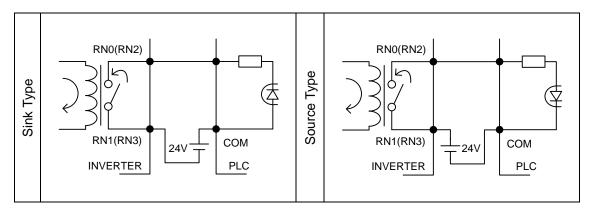
Fig 2-7 Output terminal and PLC connection
