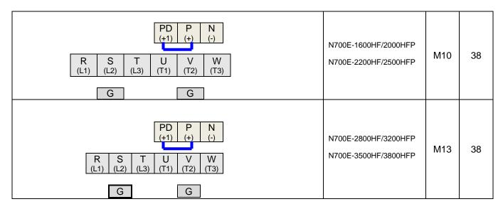
Table 2-3Wiring of main circuit terminals
