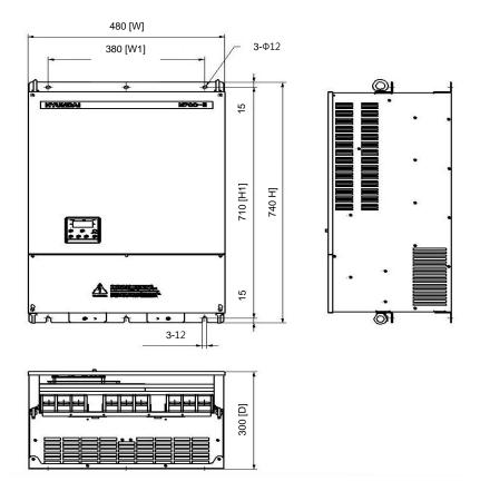
(7) N700E-1600HF/2000HFP, N700E-2200HF/2500HFPmodel external dimension.(mm)
