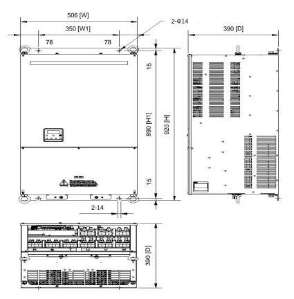
(8) N700E-2800HF/3200HFP, N700E-3500HF/3800HFPmodel external dimension.(mm)
