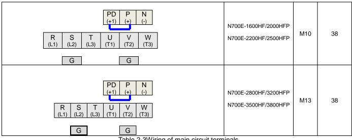
Table 2-3Wiring of main circuit terminals
