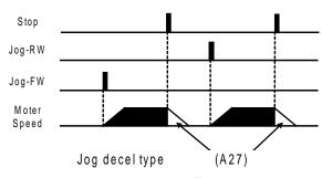
0:Free-run stop 1:Deceleration stop 2:DC injection braking
