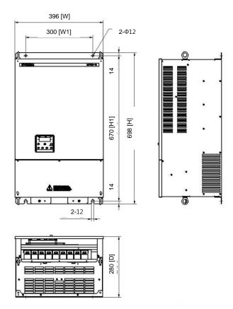
(6) N700E-1100HF/1320HFP, N700E-1320HF/1600HFP model external dimension.(mm)
