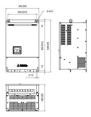
(5) N700E-750HF/900HFP, N700E-900HF/1100HFP model external dimension.(mm)
