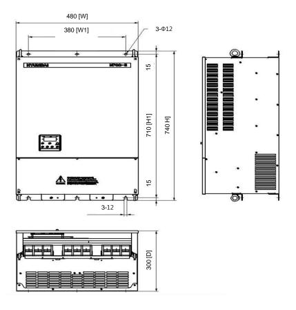
(7) N700E-1600HF/2000HFP, N700E-2200HF/2500HFP model external dimension.(mm)
