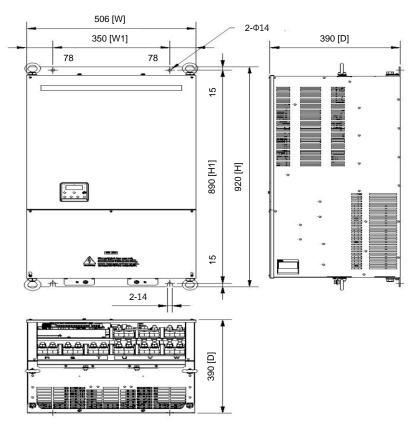
(8) N700E-2800HF/3200HFP, N700E-3500HF/3800HFP model external dimension.(mm)
