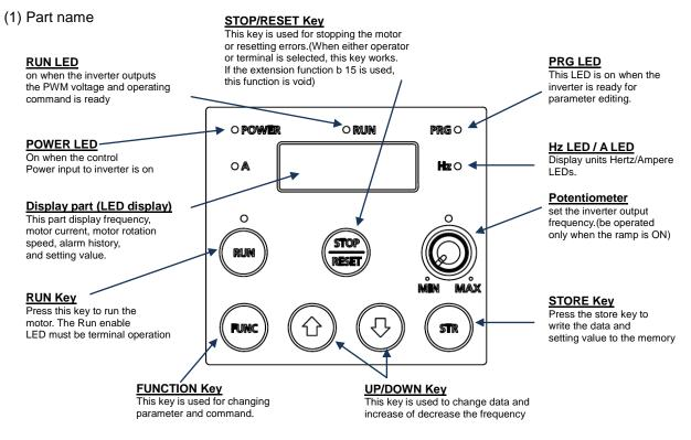
Fig.4-1 LED Type Digital Operator
