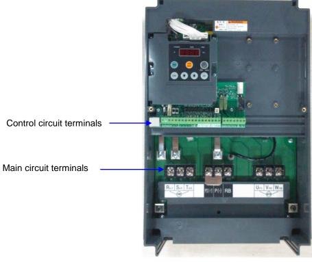
Fig1-4 Front cover removed
