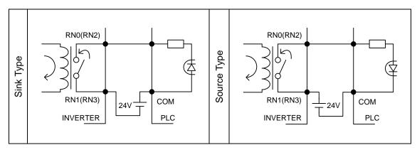
Fig 2-7 Output terminal and PLC connection
