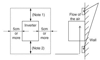
Ensure proper spacing for ventilation to prevent the unit from overheating.
