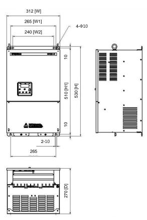
(4) N700E-450HF/550HFP, N700E-550HF/750HFP model external dimension.(mm)
