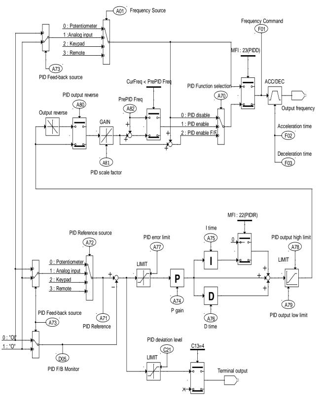
Fig4-1 PID diagram
