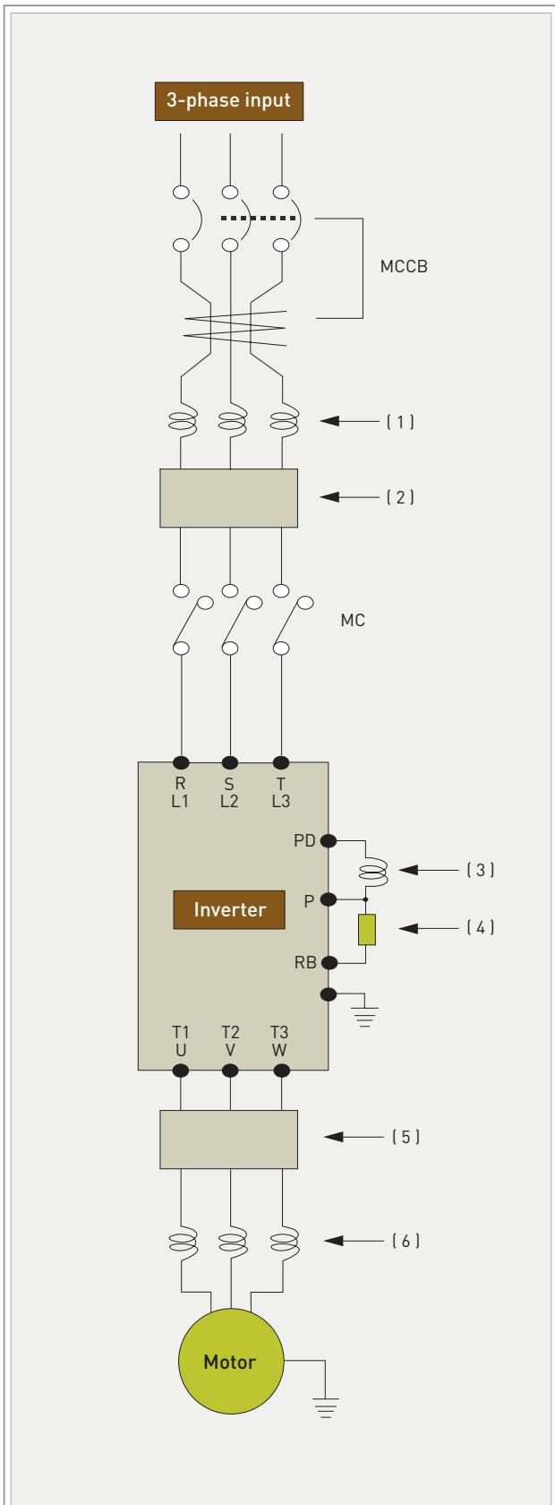
Correct selection of peripherals is required in order to normal operation of inverter
