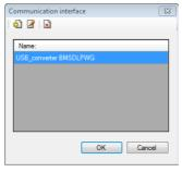
By click on the icon "New communication interface" the new converter can be add and set. Icon "Edit communication interface" allows to modify existing converter settings. By icon "Remove communication interface" the converter can be removed from the PMS professional software.
