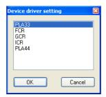
Select the appropriate instrument from the list and confirm by pressing the button OK. Then the device will be added to the list. Now it is necessary to define the ID of device in RS485 bus and communication interface used for connection to PC. Once it is done confirm setting by click on button OK.
